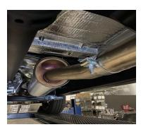
2. To remove the stock exhaust loosen the clamp from the back of the resonator. Then remove the spare tire and heat shield to aid in removal. Disengage the welded hanger using WD-40 from the OEM rubber grommets. Do not damage or remove the rubber grommets as you will reuse it to mount your new system.
